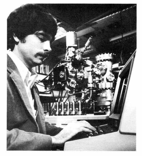
GARY KELLOGG (5114), co-developer of the pulsed-laser atom-probe, sends instructions to the computer that determines the chemical identity of atoms or molecules removed from the end of a sample shaped like a needle. The pulsed-laser
